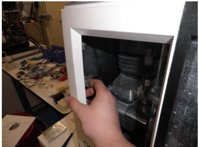
4. If full access is desired, fully open the lid and latch it in the highest position and turn the main plate locking handles counter-clockwise until the main plate locking screws disengage.
