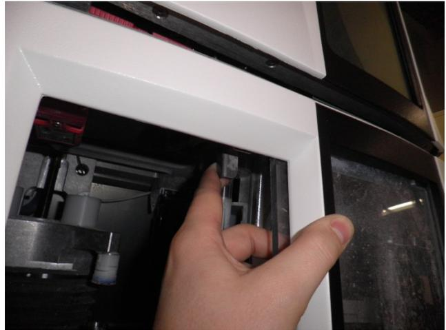
2. Disengage the service door latch and fully open the service door to access to the cutting chamber.
