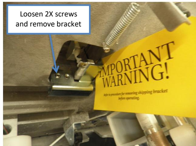
9. If the edger is equipped with a drill, it will be secured in one of two different ways.
