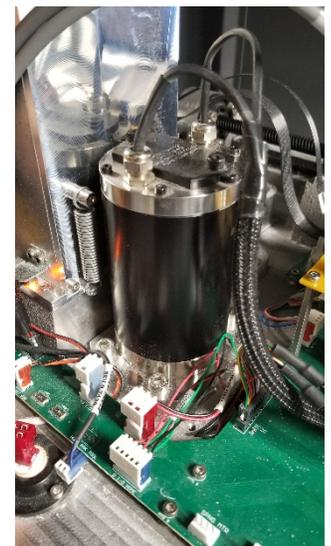
5. Pull the spindle up and out of the main plate. Pull the spindle straight up and out. If it does not come easily, rotate the spindle body back and forth as you pull up.
