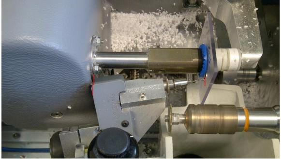
The drill assembly with drill bit will be centered between the chucked pattern blank and the cover over the axis gearbox. (SEE Next page).
