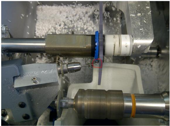
Using the 7E "Diagnostic Screen," one must move the Bevel and Size carriages into position as shown in the photo below. At some point the carriages must be moved manually and the machine needs to remain on and on the Diagnostic screen.
