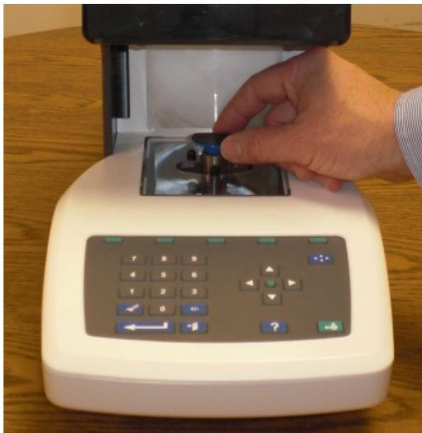
4. Press the Move button on the keypad (or press the Foot Switch on blockers that are equipped with Foot Switches). This moves the Block Holder over to the side.
