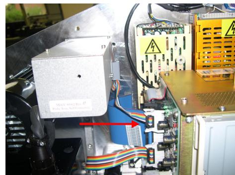
3. Using a 3/32-inch hex wrench, remove the two screws that secure the probe C-body to the probe arm. Then remove the C-body.
