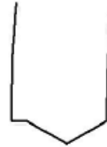
Bevel too far back -- move forward by positive bevel adjustment.
