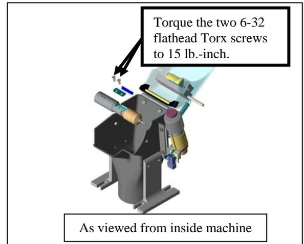
4. Remove the clamp. If you have trouble getting it to fall out, insert the end of the Torx wrench into the holes where the screws had been and lift the clamp out. Note that the rounded-off end is on the right side—you will place it back in the same way in Step 9.
