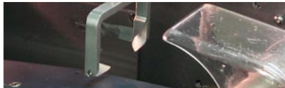
Probe in Correct Position—Note that the tips are straight down, not slanted as shown below.
