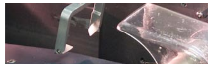
Probe in Incorrect Position—Note that the tips are slanted, not straight down.
