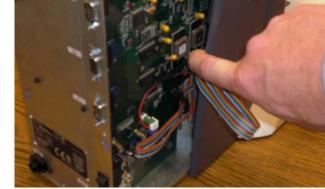
shipped in. If for any reason your blocker needs to be reverted to the prior firmware version, this chip can be re-inserted using these instructions.
