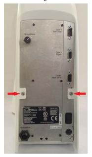
3. Gently disengage and remove the cover by pulling it out and upwards.
